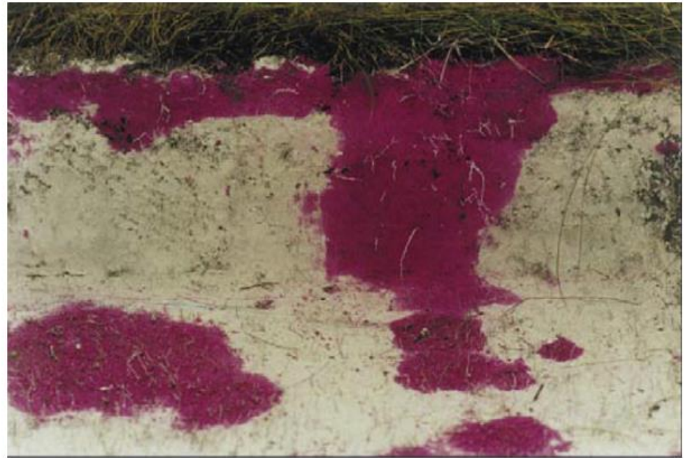
Fig. 1. Preferential flow paths in water repellent dune sand visualized by using dyestuff staining, from Dekker and Ritsema (2000).
